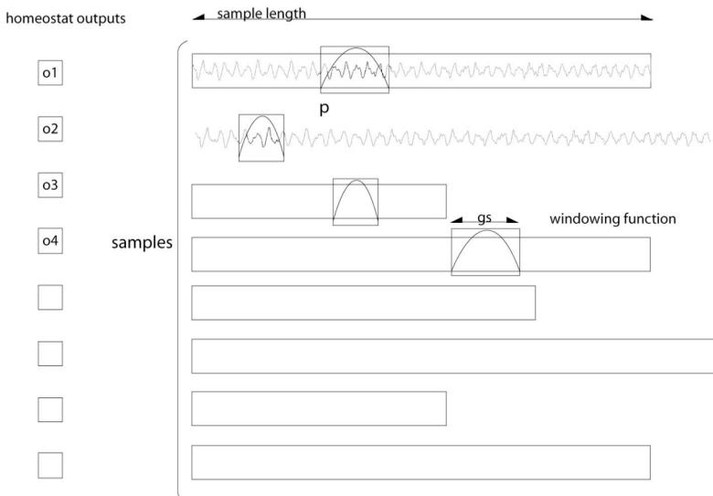
Figure. ii The outputs ( $O_n$ ) of the homeostat are used to determine to point P in the sample that grain is taken from.
